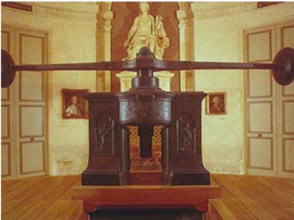
An early coining press similar to the one Mestrelle would have used, this one is hand driven, whereas Mestrelle's was reputed to be horse driven.
