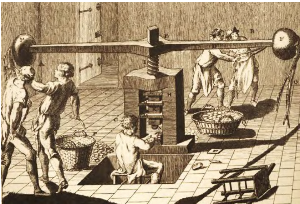
Image 2: The Balancier, a variation on the screw press, adapted for coining. It was the height of technology until replaced by the steam driven coin press in the early 19th century.
