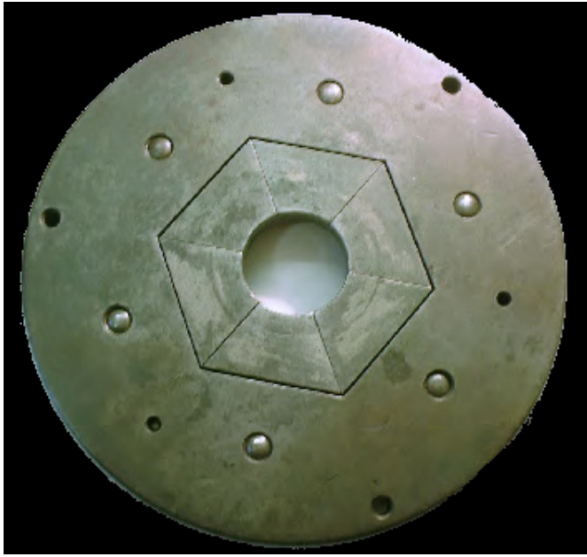
Image 3: Top view of Droz's virole brisée. Note the six sections. 4
