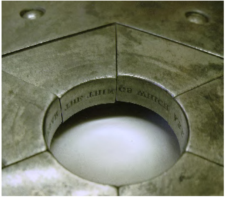
Image 4: internal view of Droz's virole brisée. Note the engraving of the individual sections.
